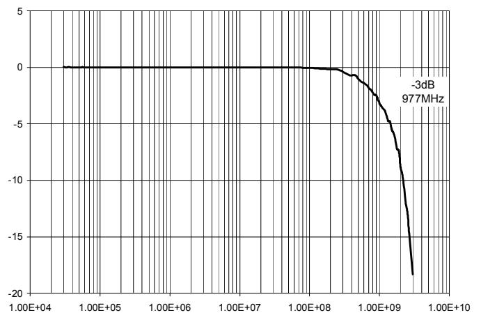
Typical Insertion Loss (S21) 30KHz to 3GHz
